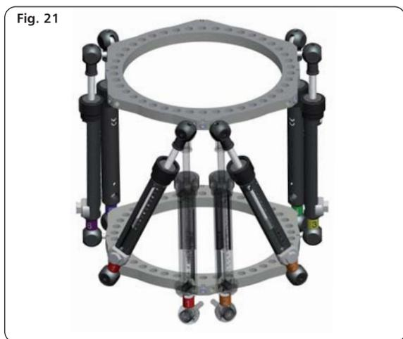
Align the anterior tab of the distal ring (anti master tab) with the master tab of the proximal ring (Fig. 21). Insert the opposite end mounting studs of struts #2 and #3 into the mounting holes of the next tab to the right relative to anterior tab. Secure the struts in place as previously instructed.
