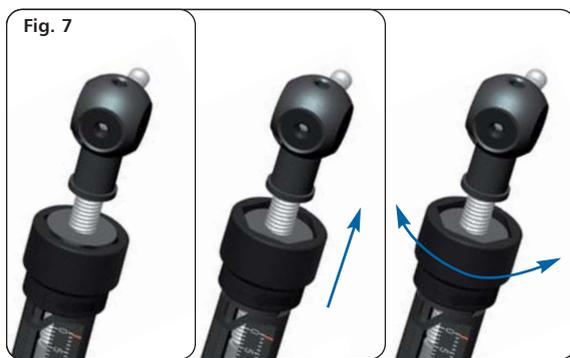
The gradual adjustment is achieved by pulling and rotating the adjustment knob resulting in a noticeable detent (click) every 0.5 mm of adjustment (Fig 7).
