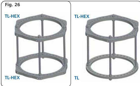
When additional stability is required, a second external support can be added to the proximal or distal rings. Since components of the TL-HEX are compatible with the TrueLok External Fixation System, external supports from the both systems can be connected to each other when building fixation blocks (Fig. 26).
