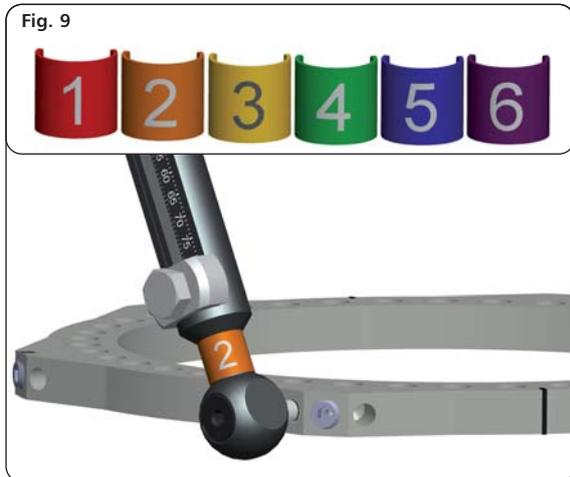
There are two types of removable aluminum strut clips: number clips to indicate the strut number and direction clips to indicate the direction of gradual adjustment. The clips are snapped on to the struts and remain in place throughout the treatment.
