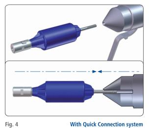
Assemble the Power Drill Torque Limiter (Check the axis and movement). (Fig. 4)
