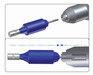
Without Quick Connection system (complete insertion into the cylindrical part)
