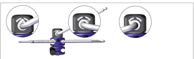
The 5mm Allen Wrench is inserted in the bolt and is turned either clockwise (3 o'clock) or counterclockwise (9 o'clock). Arrows identify the direction for moving the drop in order to engage the cam for final tightening.
