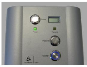
On the front of the FITBONE® Control Set, the switch labelled "Doctor" lights up blue when pressed.
