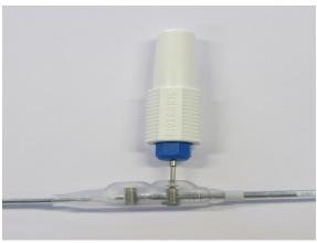
Press and turn the supplied torque wrench through the sealing lip to access the threaded pin.
