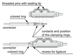
Make the connection between the connector and coupling as short as possible to prevent the bipolar feed line from kinking. On the connector for the bipolar plug connection, there is a white ring to aid with positioning. Insert the connector into the coupling until the coloured ring touches the coupling. Only then is it ensured that the contacts on the connector are positioned correctly in the coupling.
