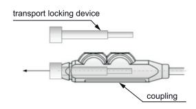
Press and turn the supplied torque wrench through the sealing lip, loosen the threaded pins and pull the transport locking device from the coupling. The transport locking device must not be turned to prevent it from breaking because fragments remaining in the bushing would prevent smooth insertion of the plug connection.
