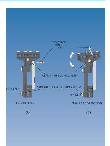
(a) shows the position of the removable locking pin of the compression-distraction unit when lengthening along the axis of the bone is required;
