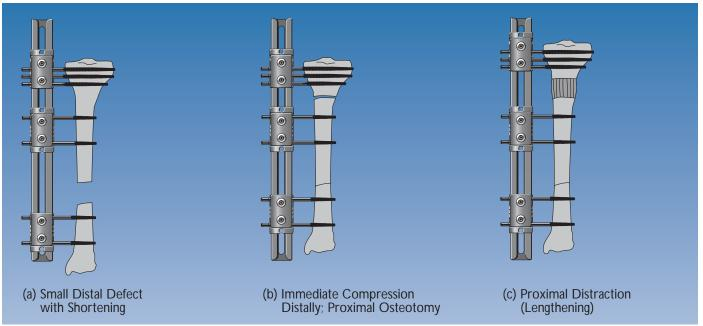
This technique is used where shortening of the limb is associated with bone loss of less than 3 cm in the tibia or 5 cm in the femur (small defect) (Saleh and Rees, 1995).
