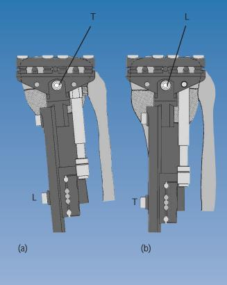
L = LoosenedT = Tightened The rail with the OF-Garches T-Clamp proximally and a straight clamp distally is then positioned, without the upper clamp cover. Once the rail has been fitted, the clamp cover is screwed tightly into place.
