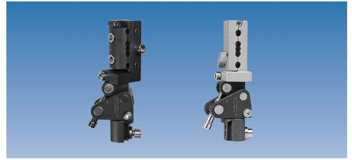
This clamp (50580) can be attached to either end of the rail, but it is not free to slide along it. It may be used for the gradual correction of angular deformity up to 70° (including translation up to a maximum of 12 mm) in any plane. It has its own template (14109) which replaces the clamp element and is attached to the angular correction element. For a description of the use of this module, see Manual 11, Part B: Correction of Deformities.
