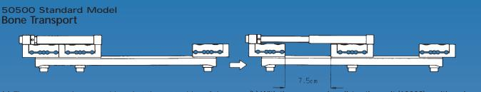
(a) The two outer clamps positioned at the extremities of the rail and middle clamp in contact with one outer clamp.
