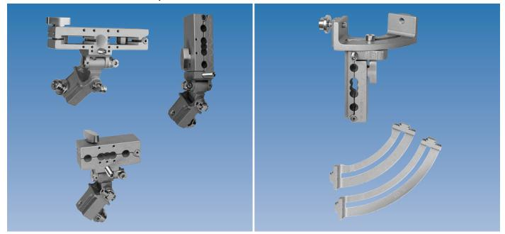
These templates, for angular and rotational correction may be attached to the rail in order to insert screws to reflect the deformity. The angular correction templates are mounted on the end of the rail but the rotational correction templates are free to slide along the length of the rail. They may be used to correct angulation in any plane or rotational deformities respectively. For a description of the use of these templates, see Manual 11, Part B: Correction of Deformities.
